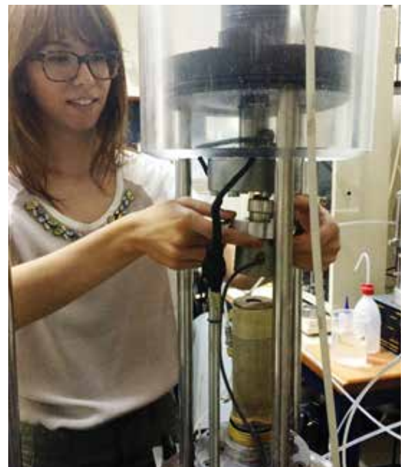
Figure 3: Antigoni Vranna, PhD candidate, prepares a cylindrical sample of stabilised sand in the cyclic triaxial device
